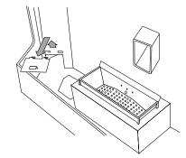
(d) Slide the ash pan trap door forward to expose the ash dumps (the door can be removed and cleaned if necessary)
